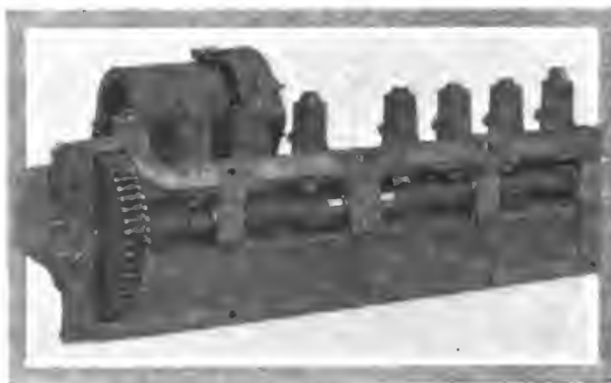
Fig. 4—Camshaft, indicating how it is placed in a separable part of the case and can be removed, with its gear, at will
